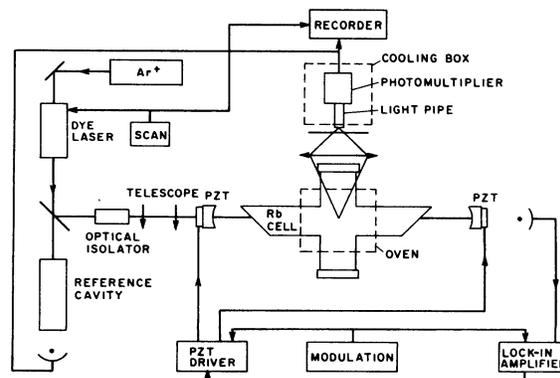
FIG. 1. Experimental arrangement.
