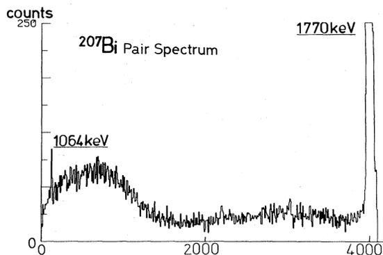
FIG. 1.  $^{207}\text{Bi}$  pair spectrum. Shown are the original photon beam energies; detected energies are 42 and 748 keV.
