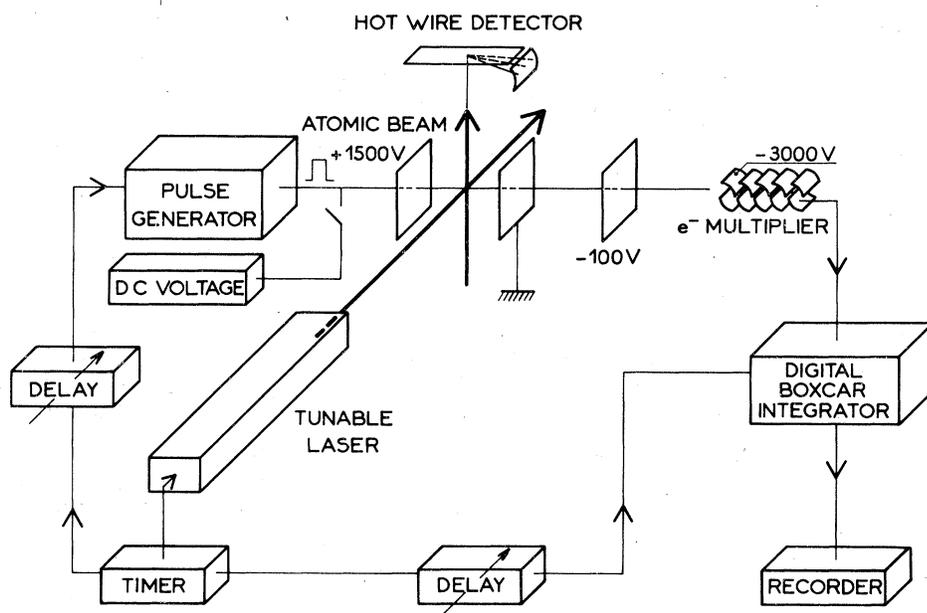
FIG. 1. Experimental set-up used for studies of Rydberg states. The tunable laser is either a nitrogen-pumped, frequency-doubled dye laser or a special pulsed single-mode source for high-resolution studies.
