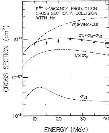
FIG. 5.  $F^{6+}$  K-vacancy production cross section in  $F^{6+}$ -He collisions as a function of the incident energy. The calculated cross sections  $\sigma_{v_1}$  and  $\sigma_{v_2}$  are described in the text.
