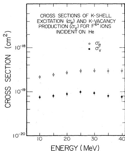
FIG. 2. Measured cross sections of single  $K$ -shell electron excitation and single  $K$ -vacancy production for  $F^{6+}$  ions incident on He.
