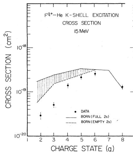
FIG. 4. Comparison between the measured and the calculated incident charge dependence of  $F^{q+}$   $K$ -shell electron excitation cross sections in  $F^{q+}$ -He collisions.
