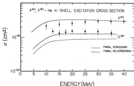
FIG. 3. Comparison between measured and calculated fluorine  $K$ -shell electron excitation cross sections in  $F^{6+}$ ,  $F^{8+}$ -He collisions as a function of incident energy.
