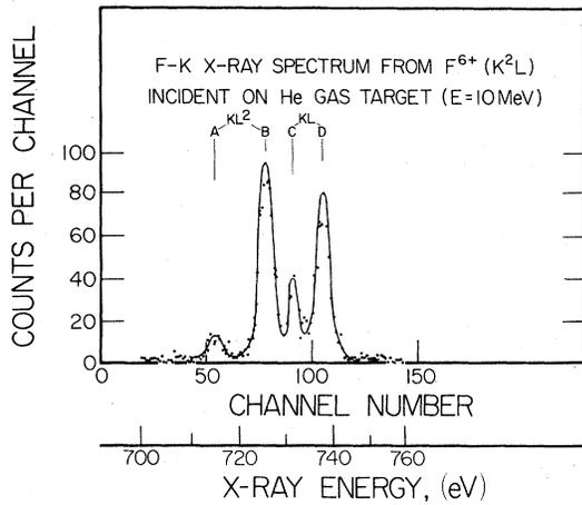
FIG. 1. A typical  $K$  x-ray spectrum from  $F^{6+}$  ions incident on He atoms. See the text for the origins of each peak.
