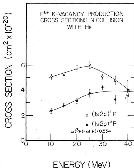
FIG. 6.  $F$   $K$ -shell vacancy production cross sections for  $F^{6+}$  ions resulting in  $(1s2p)^1P$  and  $(1s2p)^3P$  states of  $F^{7+}$  in  $F^{6+} + \text{He}$  collisions. The solid line is drawn to guide the eye.
