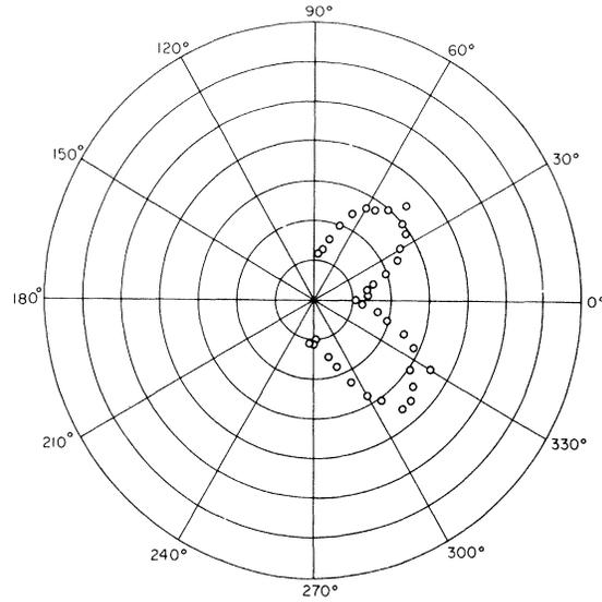
FIG. 14. Crossed-polarizer signals. The angle is that which is between the incident polarizer and the magnetic field.
