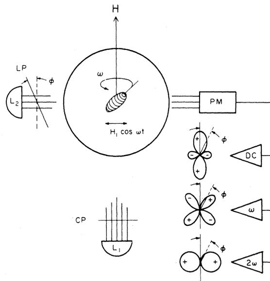
FIG. 12. Experiment on birefringence of Rb vapor.
