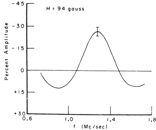
FIG. 11. Frequency analysis, illustrating the precession of positive muons stopped in aluminum with  $H=94$  G. The percent amplitude of a frequency component  $\nu$  is plotted versus frequency.
