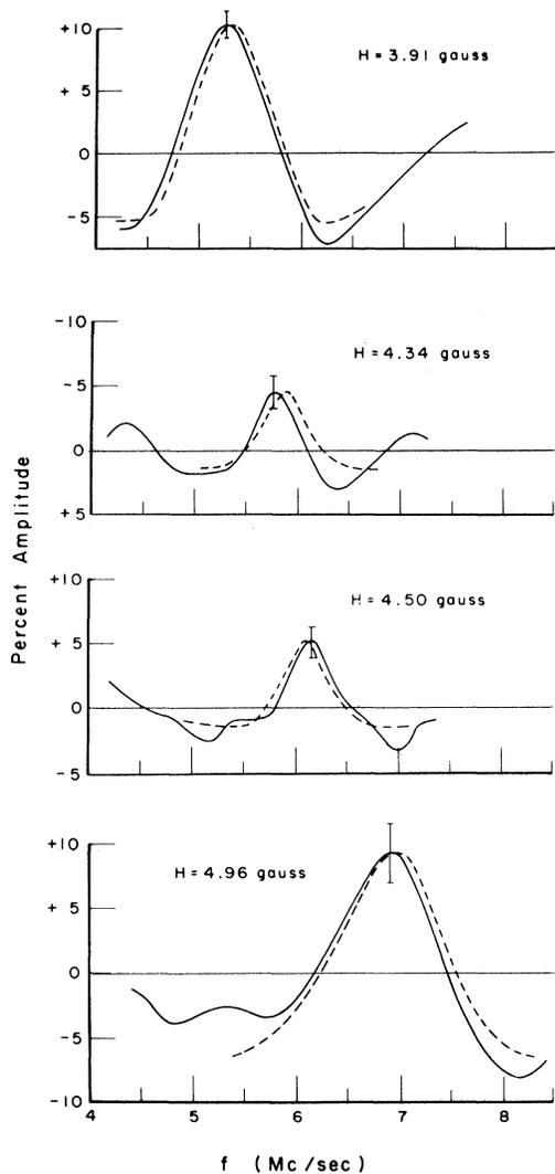
FIG. 12. Frequency analysis, illustrating the precession of muonium when polarized muons are stopped in argon gas for several magnetic-field values  $H$ . The percent amplitude of a frequency component  $\nu$  is plotted versus frequency.
