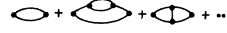
FIG. 2. The leading terms in the mass operator, written in terms of \bar{G} , the monochromatic propagator. This propagator is represented by thin lines, and the heavy dots represent gD . These three diagrams are named g^2\Sigma^{(2)} , g^4\Sigma^{(4b)} , and g^4\Sigma^{(4c)} .
