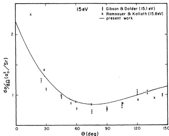
FIG. 2. Differential cross sections for the scattering of 15-eV electrons from helium. (See caption to Fig. 1 for identification of the data.)
