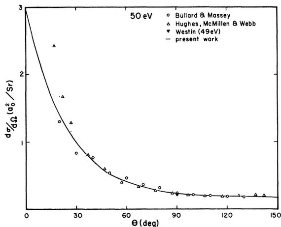
FIG. 3. Differential cross sections for the elastic scattering of 50-eV electrons from helium. The experimental point by Westin is from Ref. 10. (See caption to Fig. 1 for identification of the remaining data.)
