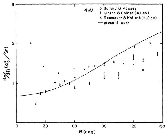
FIG. 1. Differential cross sections for the scattering of 4-eV electrons from helium. The solid curve is the result of the present extended-polarization-potential calculations. The experimental data are from Bullard and Massey (Ref. 8), Gibson and Dolder (Ref. 4), and Ramsauer and Kollath (Ref. 7).
