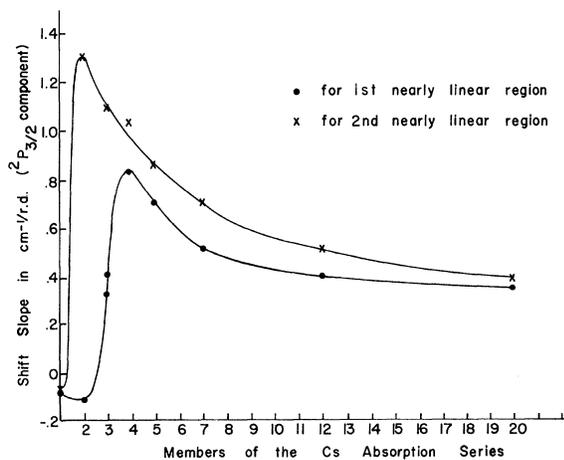
FIG. 8. Slopes of the shift versus rd (Ne) curves for the  ${}^2P_{3/2}$  components of various series lines: ● for the initial nearly linear region; × for the second nearly linear region. This graph supersedes Fig. 7 of Paper IV.
