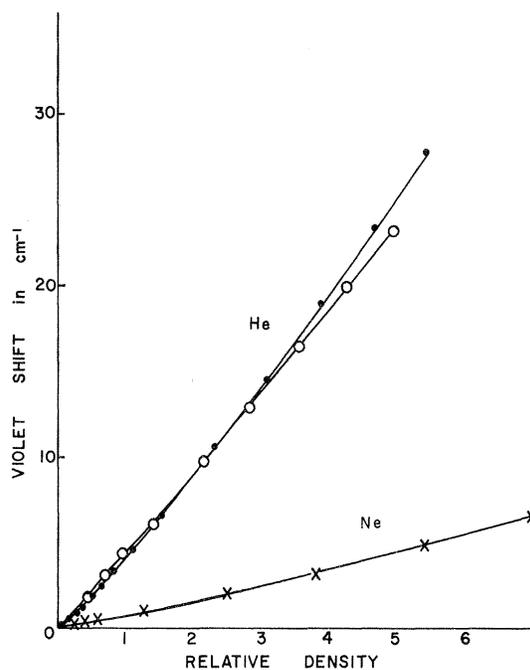
FIG. 4. Violet shift of Cs(4) produced by He ( $T = 474\text{--}523^\circ\text{K}$ ).  $\circ$  and  $\bullet$  are for  $^2P_{1/2}$  and  $^2P_{3/2}$  components, respectively. The result for Ne is reported from Paper IV for comparison.
