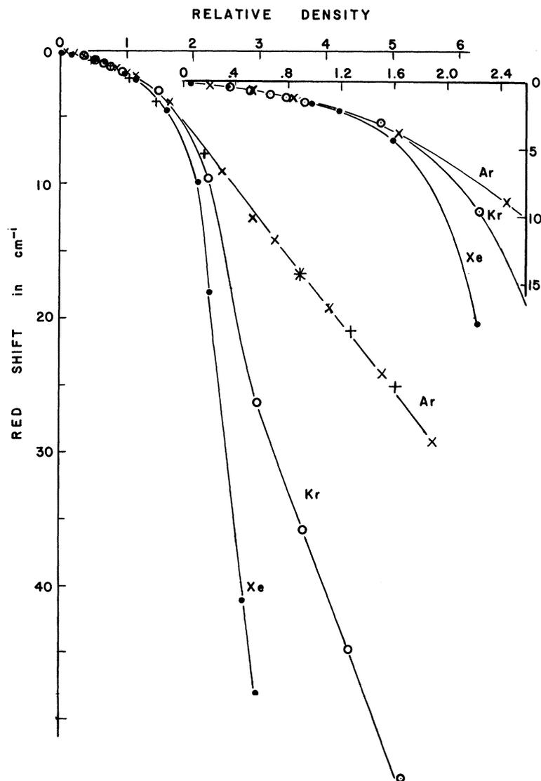
FIG. 1. Red shift of Cs(3) produced by Ar ( $T=453-512^\circ\text{K}$ ), Kr ( $T=458-508^\circ\text{K}$ ) and Xe ( $T=493-537^\circ\text{K}$ ). + and x for Ar  $^2P_{1/2}$  and  $^2P_{3/2}$  components, respectively; o and • for Kr and Xe, respectively, (for the  $^2P_{3/2}$  component only). The insert at the upper right corner is an enlargement of the plot for low rd.
