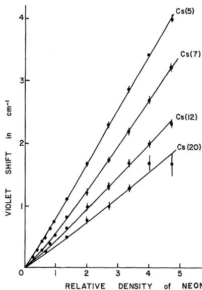
FIG. 7. Violet shift of some high-member lines by Ne ( $T = 550^\circ\text{K}$ ). Note that the shift for lower-member lines is greater than that for higher-member lines.
