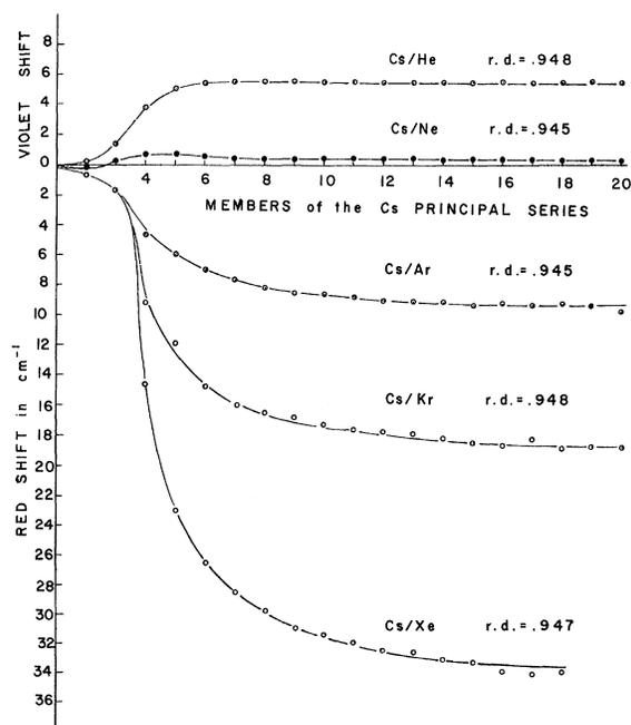
FIG. 9. Plots of the shifts versus series members for various gases at nearly the same rd and temperature ( $T=277^\circ\text{C}$ ).
