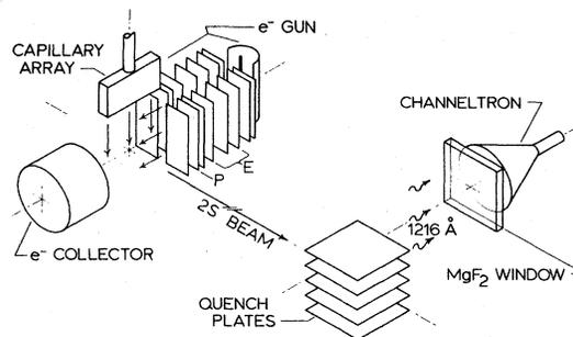
FIG. 1. Schematic apparatus diagram. The pulsed grid in the electron gun, consisting of a fine mesh covering a vertical slit, is labeled P; a three-element einzel lens is labeled E. The vertical molecular beam is shown intersecting the horizontal electron beam. The quench plates are described in Ref. 17.
