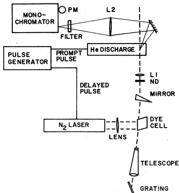
FIG. 1. Schematic diagram of the experimental apparatus. A  $N_2$  laser pumps a dye laser. The dye-laser radiation, after attenuation by a neutral-density filter, ND, is focused by a lens  $L_1$  onto the center of the He discharge. The focal region is imaged onto the entrance slit of the monochromator by a second lens  $L_2$ . A dye filter blocks scattered 388.9-nm dye-laser light while permitting the 706.5-nm fluorescence to enter the monochromator and photomultiplier tube PM.
