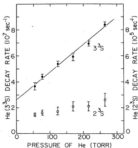
FIG. 2. Decay rates of the He  $3^3S$  and  $2^3S$  levels as a function of discharge-tube pressure. A least-squares fit of the He  $3^3S$  decay rate to the equation  $a + bP$  gives  $a = (2.63 \pm 0.20) \times 10^7 \text{ sec}^{-1}$  and  $b = (2.12 \pm 0.11) \times 10^5 \text{ Torr}^{-1} \text{ sec}^{-1}$ . The error bars represent one standard deviation in the mean decay rate at each pressure.
