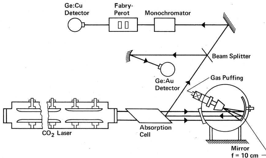
FIG. 1. Schematic diagram of CO<sub>2</sub>-laser-gas-target and backscatter optical geometry.
