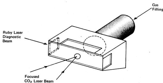
FIG. 2. Close-up view of the free-jet gas target. CO<sub>2</sub>-laser focus is approximately 3 mm inside the iris.
