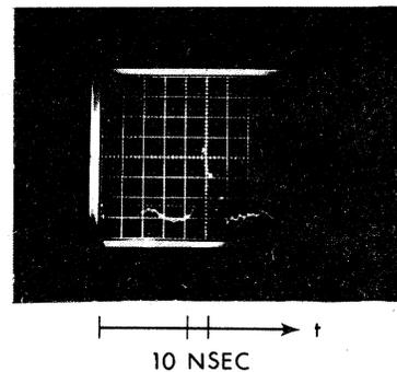
FIG. 3. Temporal structure of  $\frac{3}{2}\omega_0$  emission.
