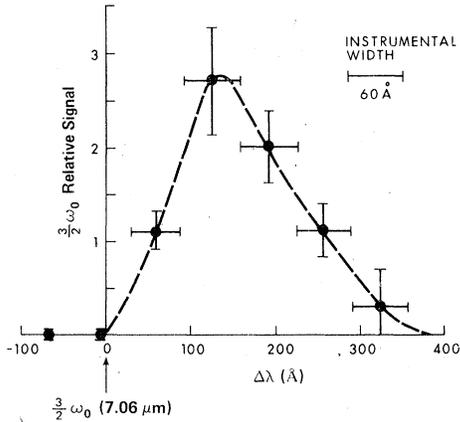
FIG. 4. Spectrum of  $\frac{3}{2}\omega_0$  emission. Data is averaged over at least six shots per point for laser intensity of  $\sim 5 \times 10^{11}$  W/cm $^2$ .
