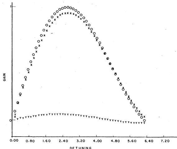
FIG. 2. Plot of the small-signal gain without space charge (open circles), space-charge reduction (Y's), and the gain including space-charge reduction (X's) for  $S=0.92$ .
