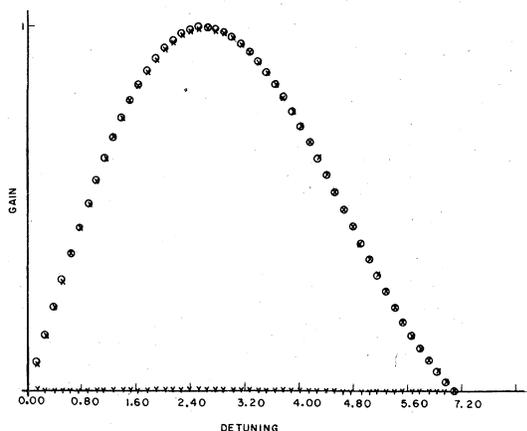
FIG. 1. Plot of the small-signal gain without space charge (open circles), space-charge reduction (Y's) and the gain including space-charge reduction (X's) for  $S=0.092$ .
