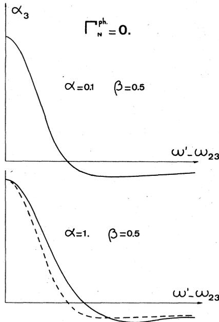
FIG. 2. Saturated absorption profiles for two values of the vcc kernel width. The dashed line represents  $\alpha_3$  in the absence of collisions, and the solid line represents it in the presence of vcc. The parameter  $\alpha$  denotes the ratio of the kernel widths of  $\Gamma_N^0/k'$ . In this figure one assumes that there is no effect of phase-interrupting collisions.
