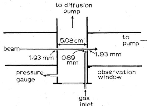
FIG. 1. Top view of a cross section of the gas-jet target.
