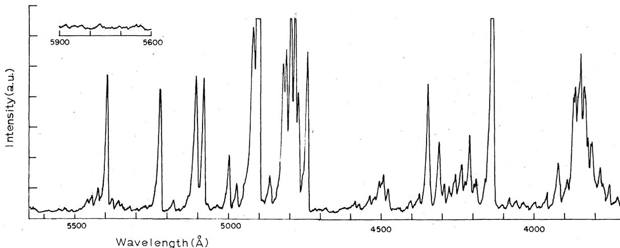
FIG. 2. Partial spectral scan of a 24.0-keV  $\text{Cl}^+$  beam taken less than 1 mm downstream from the exit aperture of the gas-jet target. The spectral window was 4.8 Å. Intensity is in arbitrary units.
