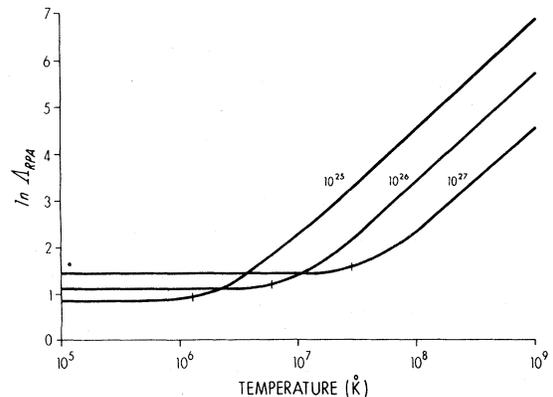
FIG. 1. RPA Coulomb logarithm as a function of temperature for different electron densities. The vertical line on each curve indicates the Fermi temperature.
