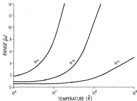
FIG. 3. Range of 3.5-MeV  $\alpha$  particles in a hydrogen plasma as a function of temperature for different electron densities. The vertical line on each curve indicates the Fermi temperature.
