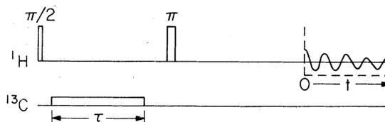
FIG. 2. Radiofrequency pulse sequence used. A  $\frac{1}{2}\pi$  pulse and a  $\pi$  pulse were applied to the  $^1\text{H}$  transitions and the resulting spin echo was recorded from time  $t=0$  for Fourier transformation. The spectrum was obtained first with no  $^{13}\text{C}$  irradiation ( $\tau=0$ ) and second with a selective  $2\pi$  pulse ( $\tau=26\ \text{msec}$ ) applied to only one  $^{13}\text{C}$  transition.
