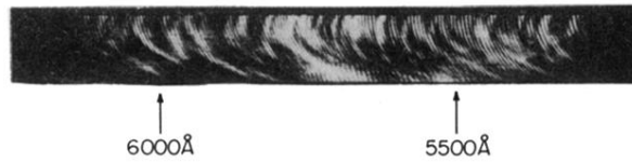
FIG. 3. Spectrogram of SB light produced in D_2O by 1.06\text{-}\mu\text{m} light. The small-scale modulation period is \lesssim 10 \text{ \AA} . Film: Polaroid 410; filtration: Corning 3-72; spectral resolution: \sim 10 \text{ \AA} .
