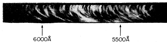
FIG. 3. Spectrogram of SB light produced in \text{D}_2\text{O} by 1.06- \mu\text{m} light. The small-scale modulation period is \leq 10 \text{\AA} . Film: Polaroid 410; filtration: Corning 3-72; spectral resolution: \sim 10 \text{\AA} .
