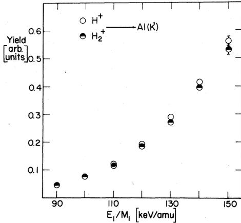
FIG. 2. Aluminum  $K$ -shell x-ray yields for projectiles  $H^+$  and  $H_2^+$  in arbitrary units vs incident energy per amu. Statistical errors are comparable to the size of points.
