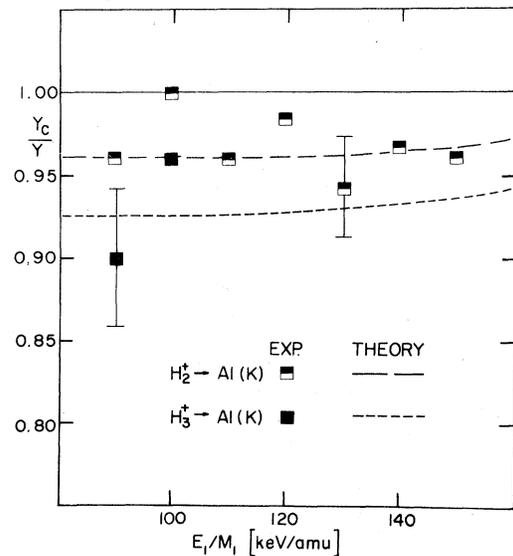
FIG. 3. X-ray yield ratios of  $H_2^+$  and  $H_3^+$  to  $H^+$ . Each point represents the average of four measurements. The curves are calculated from Eq. (5).
