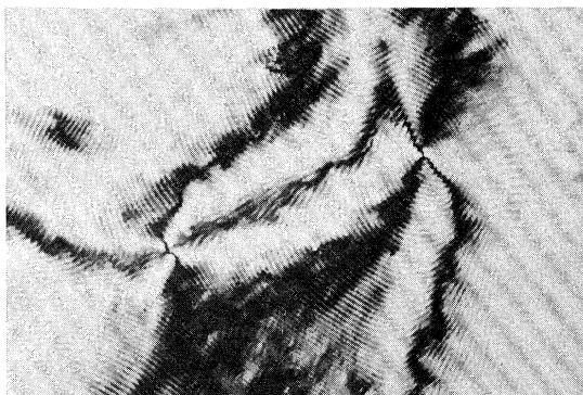
FIG. 1. Smectic C Schlieren texture with undulation lines. \bar{5}\text{BA6} , 52.7^\circ\text{C} , 133\times , crossed polarizers.
