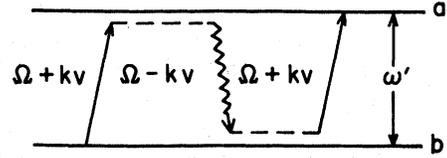
FIG. 2. Diagram showing a "three-photon absorption." There is absorption of two photons of one of the traveling waves and stimulated emission involving one photon of the other traveling wave leading to an overall net absorption. The frequency  $\omega'$  is one of the "dressed-atom" frequencies given by Eq. (12).
