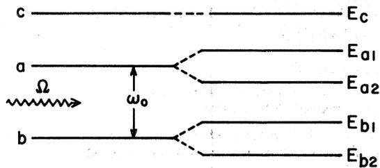
FIG. 1. A strong traveling-wave optical field with frequency  $\Omega$  in near resonance with the  $b$ - $a$  transition effectively splits each of the levels  $a$  and  $b$  into two separate levels.
