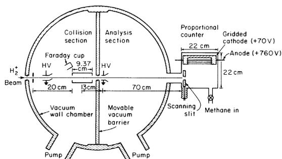
FIG. 1. Schematic diagram of the experimental apparatus.
