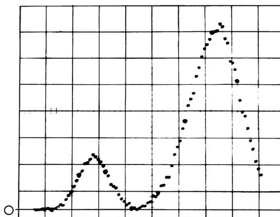
FIG. 2. Typical pulse-height distribution (100 channels) of detector-output pulses for 10-keV primary  $\text{H}_2^+$  ions, with the detector slit centered on the beam axis. The predominant peak is due to 10-keV  $\text{H}_2^+$  and  $\text{H}_2$ , and the smaller peak is due to 5-keV  $\text{H}^+$  and H, the dissociation fragments.
