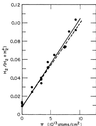
FIG. 3. Plot of fractional H<sub>2</sub> yield vs target thickness  $\pi$  for 15-keV H<sub>2</sub><sup>+</sup> in xenon. ●, data points; —, simple least-squares fit; ---, least-squares fit with attenuation correction.
