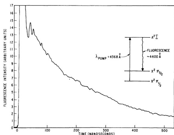
FIG. 4. Boxcar output when laser was operating at 4368 Å. The scattered laser light is clearly visible as the large off-scale spike. The laser-induced fluorescence is seen as the long, relatively slowly decaying tail. The pumping scheme is shown as an inset.
