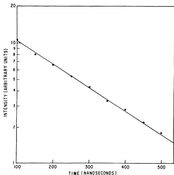
FIG. 5. Semilog plot of fluorescence intensity vs time; data points were taken from Fig. 4. The lifetime for this run was determined to be 220 nsec.
