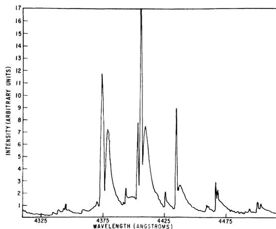
FIG. 6. Spectrum of microwave discharge of SiF<sub>4</sub>. This emission is due to the SiF  $A^2\Sigma \rightarrow X^2\Pi$  system.
