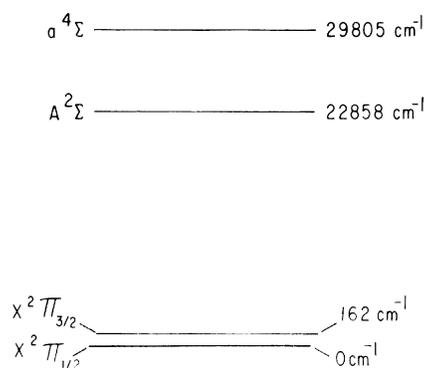
FIG. 1. Lower-lying electronic energy levels of SiF. The potential chemical laser transition is between the  $a^4\Sigma$  and  $A^2\Sigma$  states.
