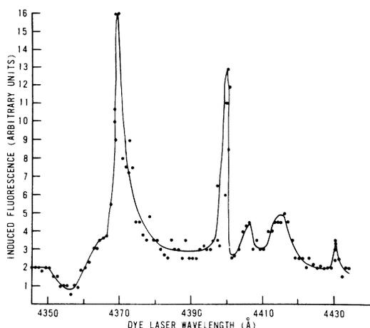
FIG. 7. Plot of the fluorescence intensity as a function of the dye-laser wavelength.
