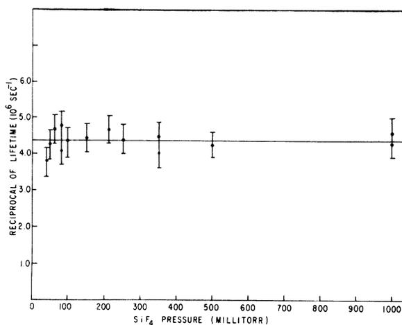
FIG. 8. Plot of  $1/\tau$  vs pressure of  $\text{SiF}_4$ . The solid line represents the average value of  $1/\tau$  for all runs regardless of  $\text{SiF}_4$  pressure.
