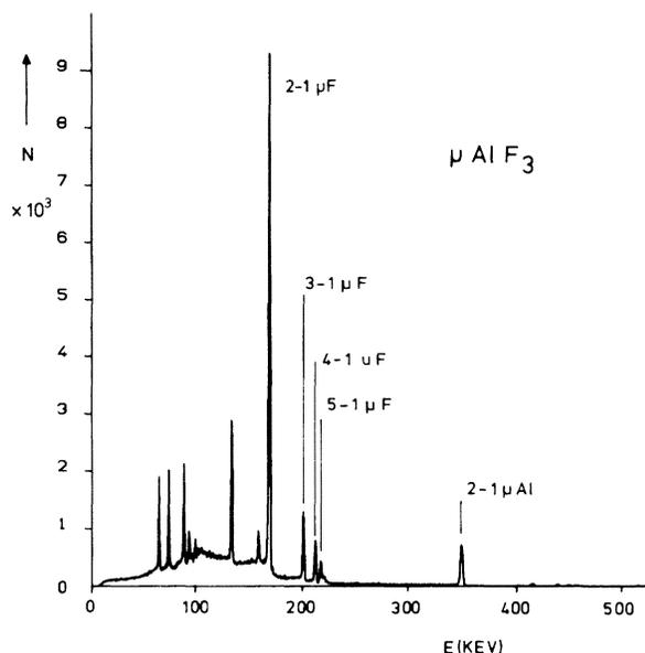
Fig. 3. Muonic x-ray spectrum of  $\text{AlF}_3$  obtained with the planar diode.
