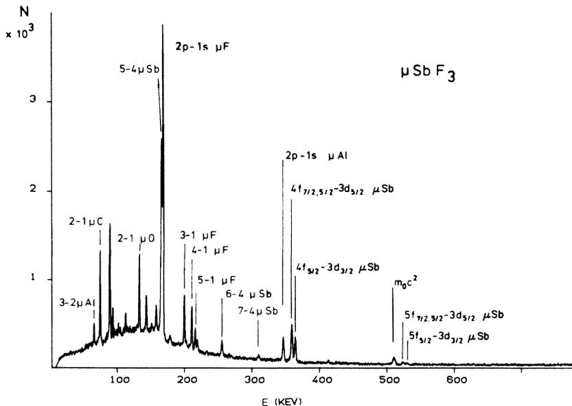
FIG. 2. Muonic x-ray spectrum of  $\text{SbF}_3$  obtained with the planar diode.
