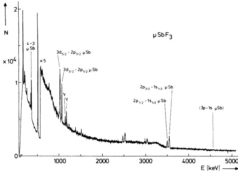
FIG. 1. Muonic x-ray spectrum of  $\text{SbF}_3$  obtained with the coaxial diode.
