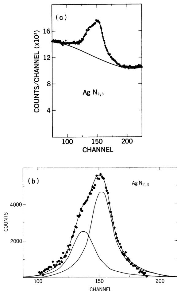
FIG. 1. Mg  $K\alpha_{1,2}$  x-ray excited photoelectron spectrum of Ag. (a) Original spectrum with smoothing and computer-fitted background. (b) Deconvolution of the background-subtracted spectrum into Lorentzian shapes produced with a DuPont 310 curve resolver, subject to the criterion that the  $N_2/N_3$  intensity ratio be  $\frac{1}{2}$ . Units on the abscissa are 0.4 eV/channel.
