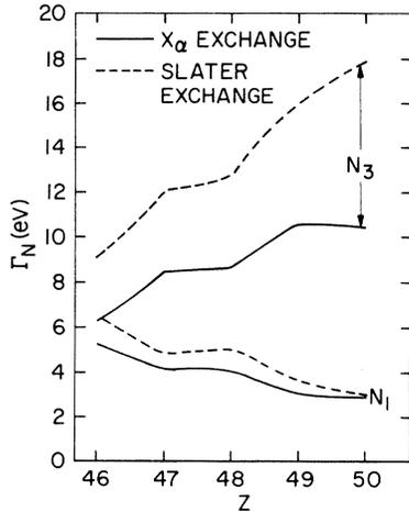
FIG. 3. Dependence of the  $N_1$ - and  $N_3$ -level widths on the choice of exchange used in the calculation, illustrating extreme sensitivity of the dominant radiationless transition rates to the atomic potential.
