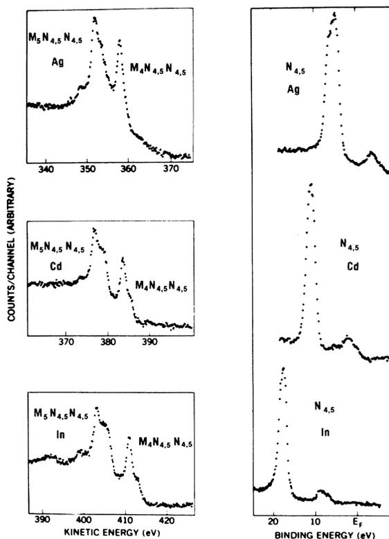
FIG. 2.  $M_4$ - $N_{4,5}N_{4,5}$  and  $M_5$ - $N_{4,5}N_{4,5}$  Auger spectra (left-hand side) and Mg  $K\alpha$  x-ray excited  $N_{4,5}$  photoelectron spectra (right-hand side) of Ag, Cd, and In. The small peak in the  $N_{4,5}$  photoelectron spectra is caused by the Mg  $K\alpha_{3,4}$  satellite radiation from the x-ray source.
