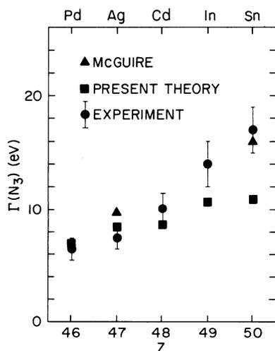
FIG. 7. Comparison of measured  $N_3$ -level widths with theoretical results from this work and of McGuire (Ref. 10).
