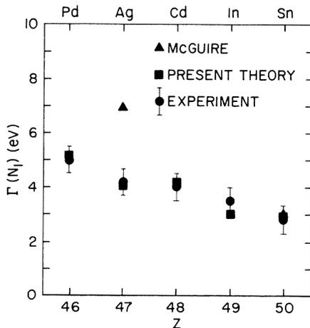
FIG. 4. Comparison of theoretical and experimental widths of  $N_1$  vacancy states. Experimental data and free-atom calculations are from the present work; triangles represent the lower of two sets of results obtained by McGuire (Ref. 10) under different energy assumptions (see text, Sec. III B 2).
