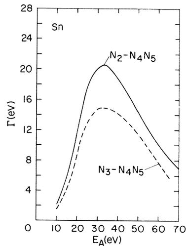
FIG. 5.  $N_2$ - $N_4N_5$  and  $N_3$ - $N_4N_5$  partial widths of Sn as functions of Auger electron energy, illustrating steep energy dependence of these super-Coster-Kronig transition rates.
