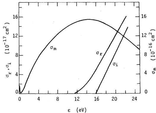
FIG. 1. Argon cross sections used in the calculations:  $\sigma_m$ , momentum transfer;  $\sigma_r$ , excitation;  $\sigma_i$ , ionization.
