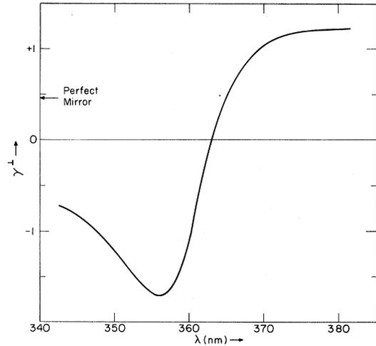
FIG. 4. Frequency-shift parameter  $\gamma^\perp$  of a perpendicular dipole embedded in a dielectric of refractive index 1.50, and centered between two silver mirrors.
