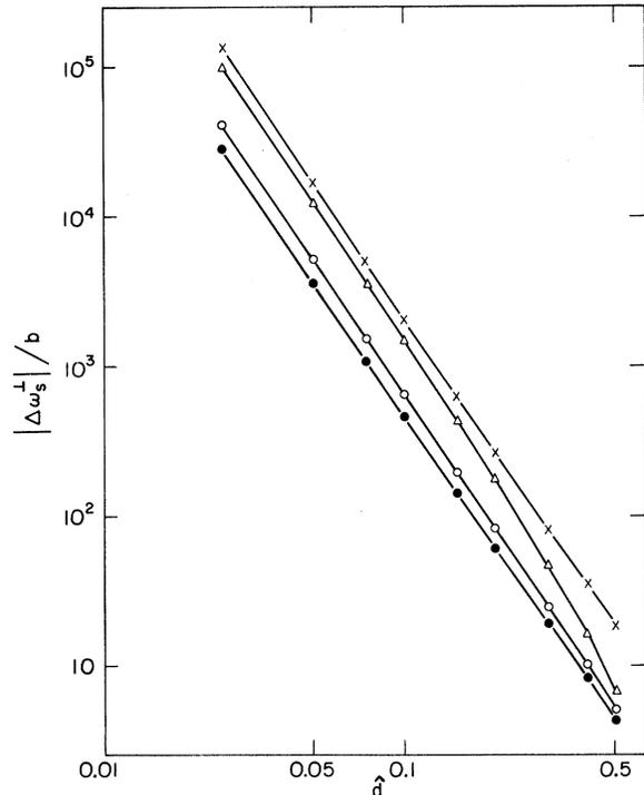
FIG. 5. Frequency shift  $(\Delta\omega_s^\perp/b)$  vs distance  $(\hat{d})$  in the small-distance region for a perpendicular dipole centered between two mirrors and embedded in a dielectric of  $n_1 = 1.50$ . The curves are for different values of the refractive indices of the metal: (x)  $\hat{n} = 0.09 + i1.476$ ; (●) perfect mirror; (Δ)  $\hat{n} = 0.05 + i1.864$ ; (○)  $\hat{n} = 0.06 + i4.11$ .
