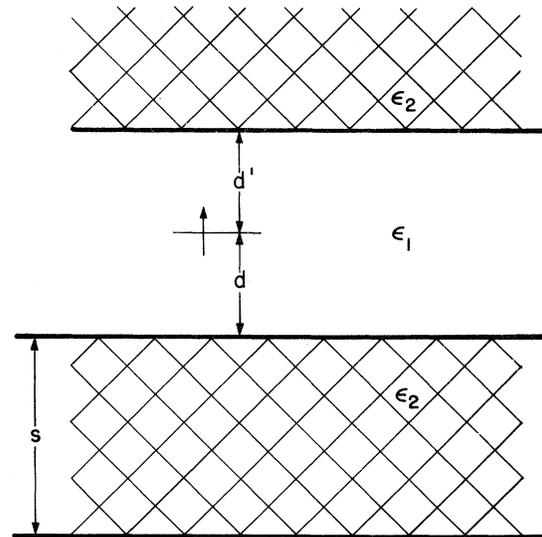
FIG. 1. Geometry of the mirror problems treated herein. The distance from the dipole to the lower partially reflecting surface is  $d$ ; the thickness of this mirror is  $s$ ; the distance from the dipole to the upper surface is  $d'$ . The first problem is a single thick mirror ( $d' = \infty, s = \text{finite}$ ); the second is a single thin mirror ( $d' = \infty, s = \infty$ ); the third problem is for double thick mirrors ( $d' = d, s = \infty$ ).
