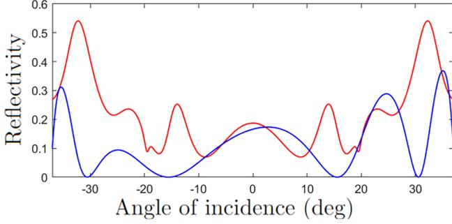
FIG. 7. Comparison between the reflectivity of gyro-uniaxial multilayer structures whose gyrotropic components are described by Eq. (1) (red symmetric curve) and Eq. (17) (blue asymmetric curve).
