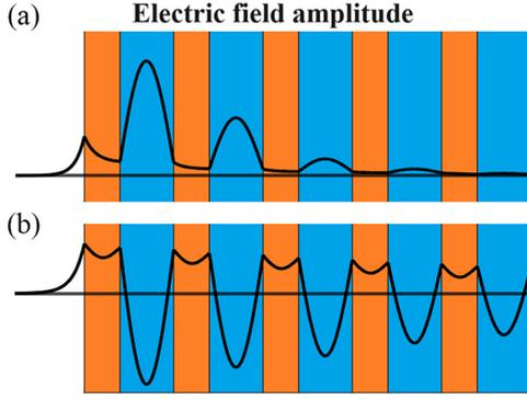
FIG. 4. Typical space distributions of the  $y$  component of the electric-field amplitude in a semi-infinite gyro-uniaxial PC. The blue regions represent the uniaxial components, whereas the orange regions represent the gyrotropic components. (a) Tamm wave. (b) Intermediate surface mode.
