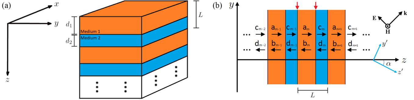
FIG. 1. (a) Outline of the one-dimensional periodic multilayer structure. (b) Outline of the  $yz$  plane section of the periodic structure under consideration. Here  $y'$  and  $z'$  represent the principal axes of the hyperbolic slabs
