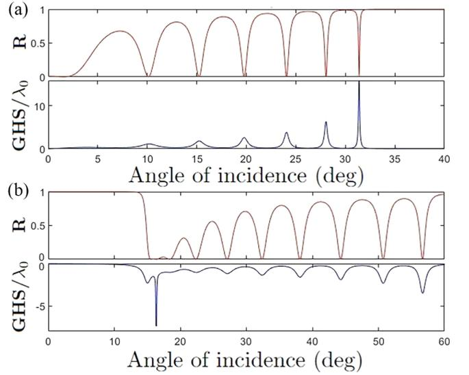
FIG. 6. Reflectivity and Goos-Hänchen shift (in units of the incident wavelength) for two multilayer structures composed of ten periods, calculated using the transfer matrix method. The structural parameters are the same as in Fig. 2. The other parameters are (a)  $\omega_{p,\parallel} < \omega_{p,\perp}$ , corresponding to forward surface modes of Fig. 2(d), and (b)  $\omega_{p,\parallel} > \omega_{p,\perp}$ , corresponding to backward-propagating surface modes of Fig. 2(f).
