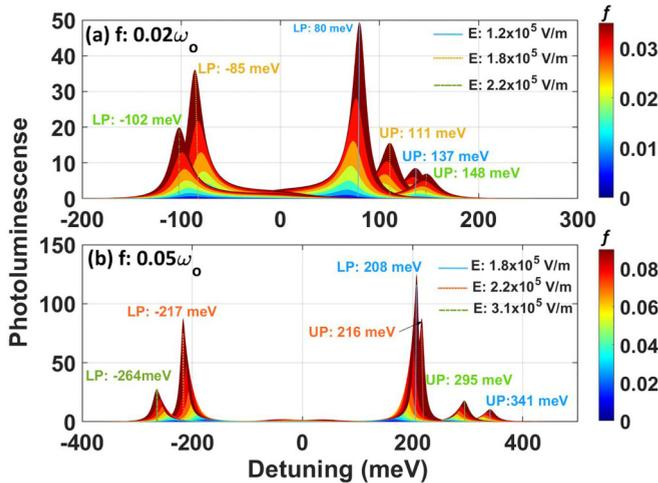
FIG. 5. Photoluminescence spectra of Stark-tuned plexcitonic states as a function of detuning ( $\Delta_m$ ) for (a)  $f = 0.02\omega_0$  and (b)  $f = 0.05\omega_0$ . UP plexciton blueshifts and LP redshifts as the Stark field strength increases.
