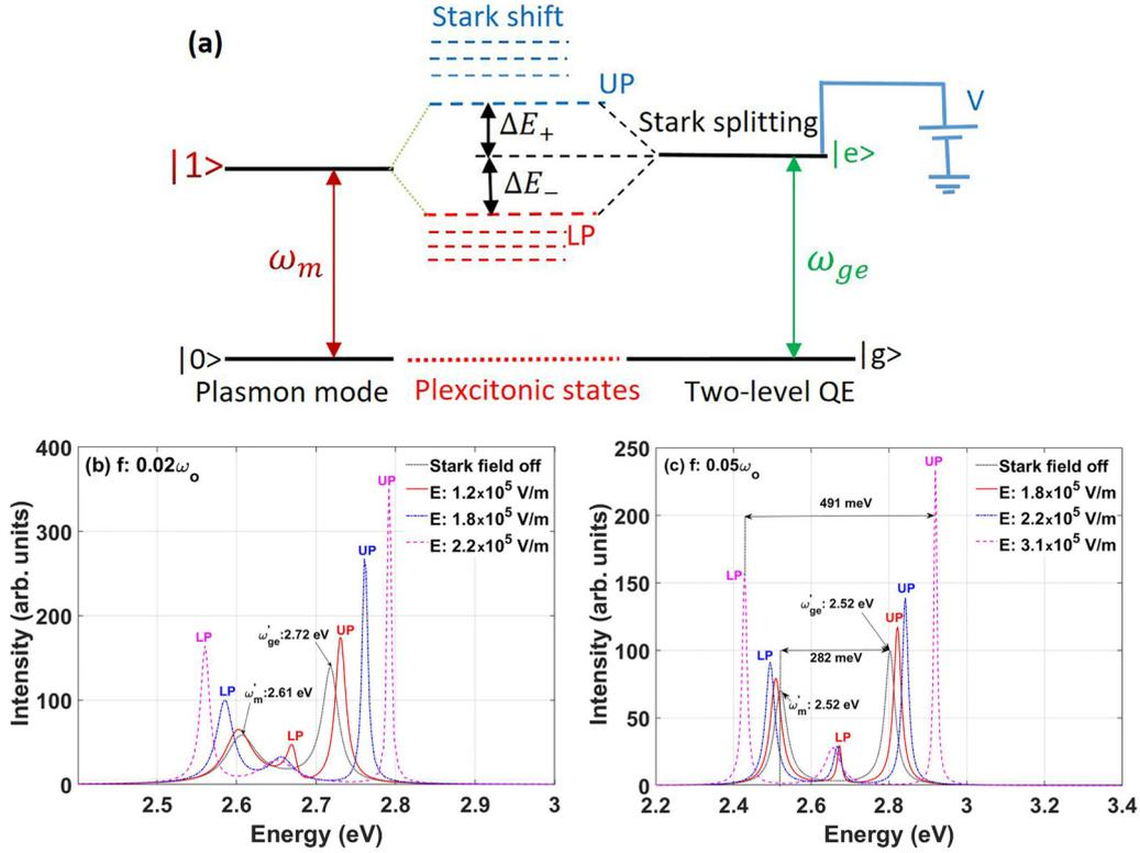
FIG. 4. (a) Schematic diagram of PM coupled to two-level QE ( $\omega_m \approx \omega_{01}$ ), and the tuning of plexcitonic states through Stark-induced splitting and shifts. Stark-tuned hybrid plexcitonic states in the resonantly coupled plasmon-emitter system for (b) weak and (c) intermediate coupling.
