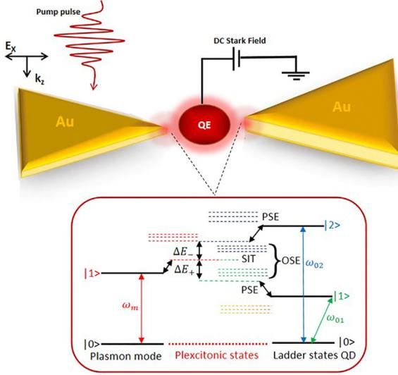
FIG. 1. Schematic diagram of a hybrid system of an Au bow-tie nanoantenna and a three-level QE. QE is attached to an external voltage bias which induces Stark shifts in the hybrid plexcitonic states.
