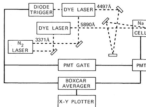
FIG. 1. Schematic diagram of the apparatus with the lasers tuned to pump the  $7d$  level via the  $3p_{3/2}$  level.
