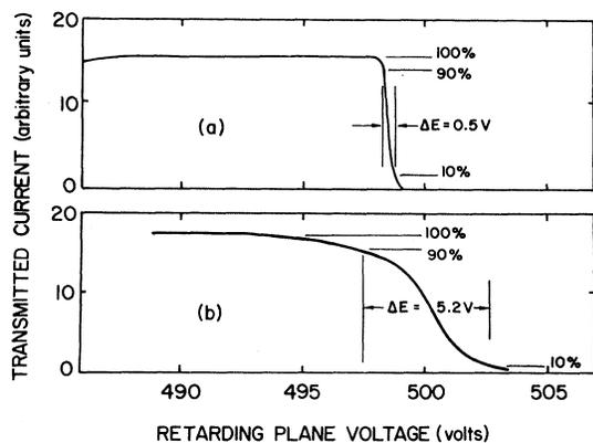
FIG. 3. Transmitted electron current through the filter lens vs retarding voltage: (a) electrons from chemi-ionization of  $\text{CO}_2$  and (b) electrons ejected from the surface of the extraction aperture by  $\text{He}(2^3\text{S})$  atoms when no reactant gas is introduced.
