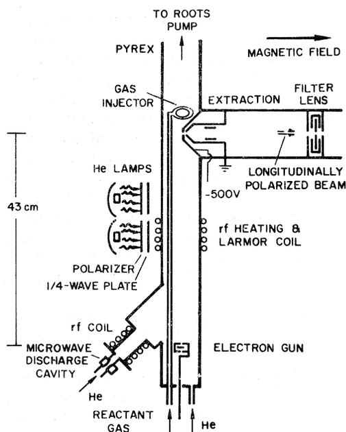
FIG. 1. Schematic diagram of the apparatus as configured to perform optimally as a source of polarized electrons (not drawn to scale).
