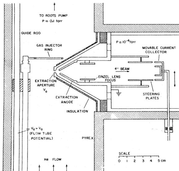
FIG. 2. Detail of the gas injector and electron extractor. The injection ring has 12 holes on the inside diameter and 28 on the outside, each 0.25 mm in diameter.
