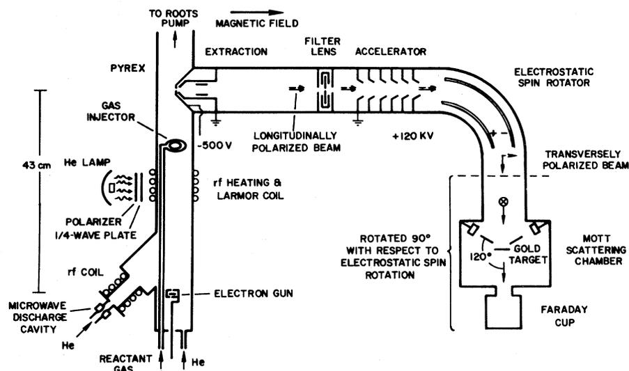
FIG. 1. Schematic diagram of the experimental apparatus (not drawn to scale).
