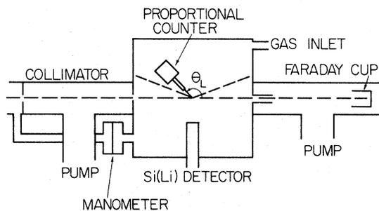
FIG. 1. Schematic diagram of the experimental arrangement.
