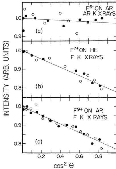
FIG. 3. Angular distributions of x rays corrected for kinematic and geometric effects as explained in the text. Closed circles:  $\theta < 90^\circ$ ; open circles:  $\theta > 90^\circ$ . The solid curves represent the best straight lines through the data. The polarization fractions  $P$  are given by the slopes of these lines: (a) target x rays:  $P = 0.028 \pm 0.030$ ; (b) projectile x rays:  $P = 0.221 \pm 0.017$ ; (c) projectile x rays:  $P = 0.234 \pm 0.014$ .
