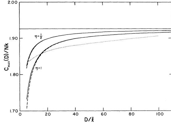
FIG. 2. Height  $C_{\max}(D)$  of the specific-heat maximum. First-order results: dashed line; second-order results: solid line. The dotted line represents the numerical results of Hasan and Goble for the case  $\eta = \frac{1}{2}$ , while the horizontal line corresponds to the bulk value  $C_0(\infty)$ .
