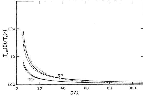
FIG. 1. Temperature  $T_{\max}(D)$  at which the specific heat of an infinite slab of thickness  $D$  is maximum. First-order results: dashed line; second-order results: solid line. The dotted line represents the numerical results of Hasan and Goble for the case  $\eta = \frac{1}{2}$ .
