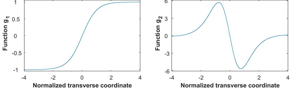
FIG. 2. Modulus of the functions  $g_1(y)$  and  $g_2(y)$ . The normalized transverse coordinate is  $y = \alpha_0 x$ , where  $x$  is the spatial coordinate  $x$  and  $\alpha_0 = (2 \tan \beta_0)/h_0$ . The wavelength is  $\lambda = 633$  nm, the reference height is  $h_0 = \lambda/4$ , and the sidewall angle is  $\beta_0 = 80^\circ$ .
