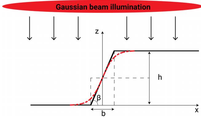
FIG. 1. Sketch of a Cliff-like nanostructure with sidewall angle  $\beta$  and height  $h$ . The red dashed line corresponds to the mathematical model of the slope. The sidewall angle  $\beta$  is related to the parameter  $\alpha$  as  $\alpha = 2/b = 2 \tan \beta/h$ .
