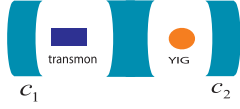
FIG. 1. Schematic of the coherent coupling system. A transmon is capacitively coupled to microwave cavity c_1 , while a magnon is coupled to microwave cavity c_2 via the magnetic dipole interaction. The two microwave cavities c_1 and c_2 are coupled via a hopping interaction. Each cavity can be a one-dimensional or three-dimensional cavity.
