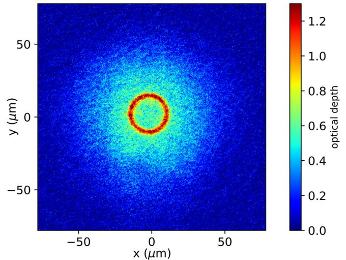
FIG. 2. Density distribution of  ${}^6\text{Li}$  atoms in our trap when the Fermi level is around 0.1  $\mu\text{K}$  larger than the depth of the dimple created by the ring-pattern beam. The plot shows the average of 10 *in situ* absorption images taken at a magnetic field of 100 mT. Both the ring-shaped region of increased density and the dilute halo are clearly visible.
