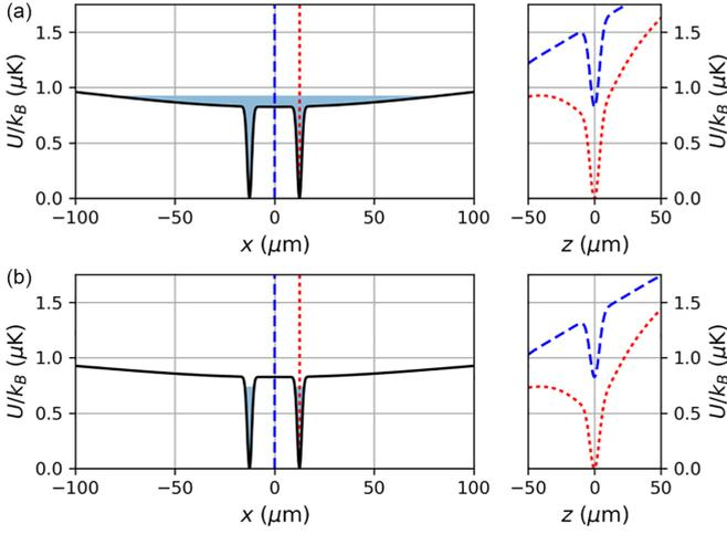
FIG. 3. Potential-energy slices of our combined trap (gravity included) for (a) 40-mW and (b) 30-mW sheet power. The left plots show the radial trap profiles at  $z = 0$ , while the right plots show the vertical profiles for two different radii: The blue dashed line is the vertical cut along  $r = 0$ , and the red dotted line is along  $r = r_0$ . The shaded regions in the radial profiles indicate where the potential energy is below the evaporation depth  $V_{\text{evap}}$ .
