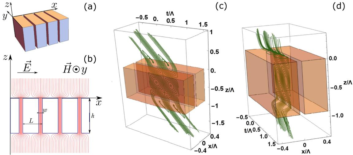
FIG. 2. (a) Slit grating, invariable in the  $y$  direction, made in a perfect conductor. (b) Time-averaged Poynting vector lines in the resonant case,  $p$ -polarized normally incident monochromatic wave. (c) ESs in the central plane of a slit. (d) ESs crossing the line  $z = -h/2, x = -2w/5$ .
