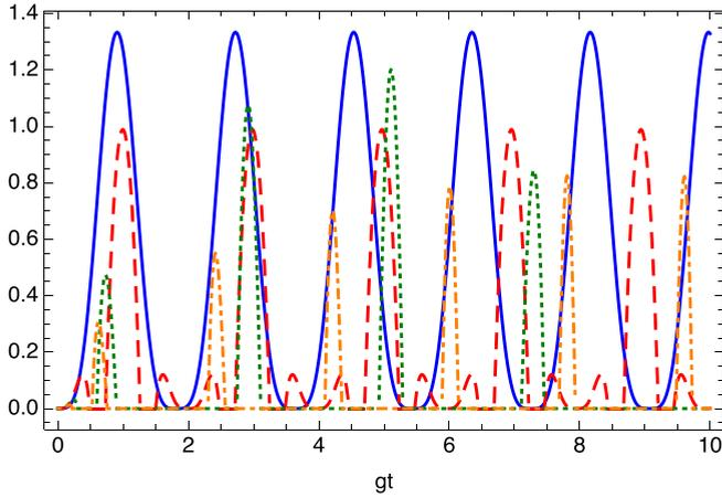
FIG. 3. Entanglement, as indicated by positive values of the left-hand sides of Eqs. (42) and (43), for a system of three atoms starting from the ground state with  $n_0 = 1$  (solid line), 2 (dashed line), 3 (dotted line), and 4 (dot-dashed line) photons, respectively. For  $n_0 = 1$ , only the left-hand side of Eq. (43) contributes (i.e., is greater than zero). For larger  $n_0$ , however, its contribution is limited to small secondary minima, here only visible for  $n_0 = 2$ .
