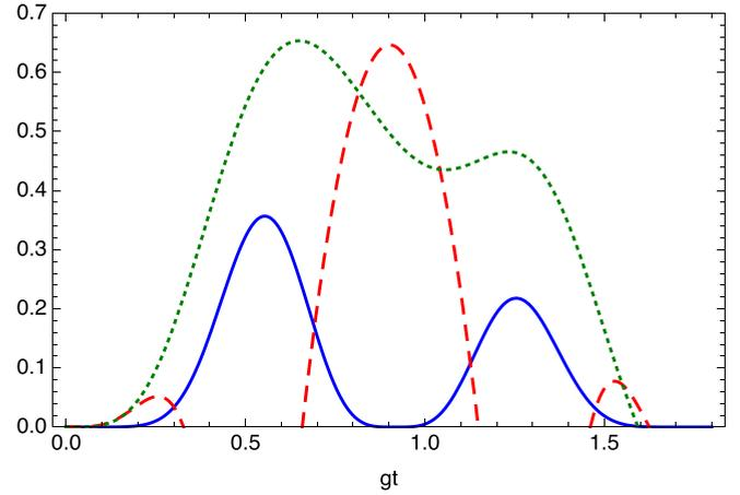
FIG. 6. Entanglement for the case  $N = 4$  and  $n_0 = 3$  as detected by inequalities (53) (solid line), (57) (bipartite entanglement, dashed line), and Eq. (52) (dotted line). Note that the solid line is actually always above zero except at  $gt\sqrt{14} = 2n\pi$ , whereas the other two cross the horizontal axis with a nonzero slope. Note also the existence of a small region to the right where the dashed line detects entanglement but the dotted one does not.
