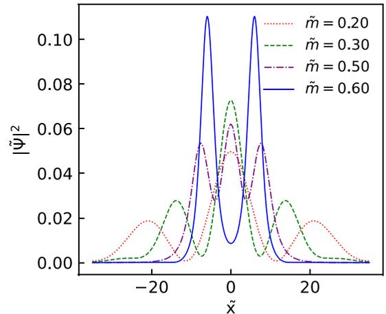
FIG. 3. Interference pattern at time  $\tilde{t} = 8.9$  for different values of  $\tilde{m}$ . The interference gets progressively less sharp as the mass increases, until it is completely suppressed.
