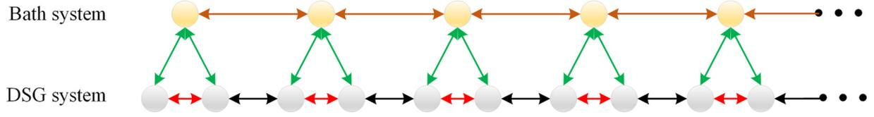
FIG. 8. The proposed setup. The red (black) arrows indicate the intracell (intercell) hopping of spin-polarized fermions in the DSG system. The brown arrows indicate the hopping of fermions in the bath, while the green arrows are the modulation between these two systems.
