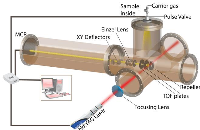
FIG. 1. Schematic of the time-of-flight mass spectrometer setup developed for multiphoton ionization and dissociation experiments.
