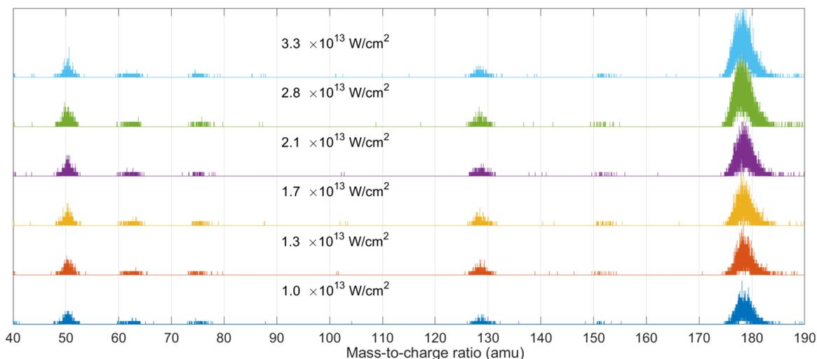
FIG. 3. Phenanthrene MPI and MPD spectra at different laser intensities. Fragments of a mass-to-charge ratio above 40 amu. A vertical offset is maintained to show spectra at different laser intensities separately.
