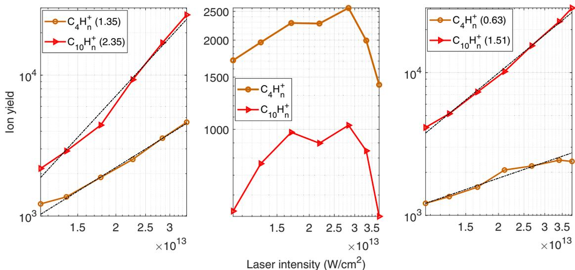
FIG. 4. Laser power dependence of the yield of  $C_4H_n^+$  and  $C_{10}H_n^+$  from anthracene (left), phenanthrene (middle), and pentacene (right). The numbers in brackets denote the slope of the fitted linear curves for each group.
