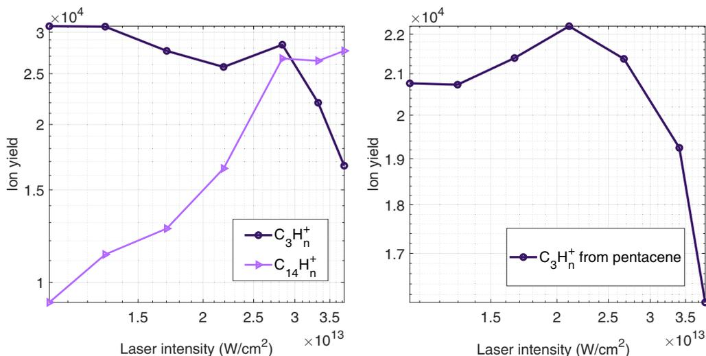
FIG. 5. Left: Laser power dependence of the yield of  $C_3H_n^+$  and  $C_{14}H_n^+$  fragments from phenanthrene. Right: Laser power dependence of the yield of the  $C_3H_n^+$  fragment from pentacene.
