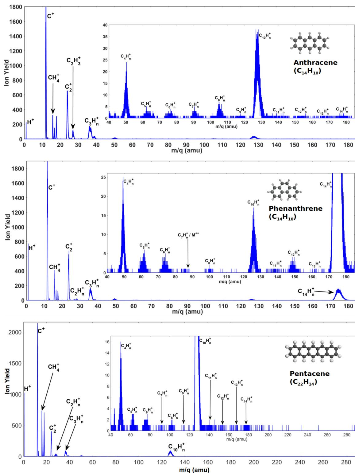
FIG. 2. MPI and MPD spectra of anthracene, phenanthrene, and pentacene
