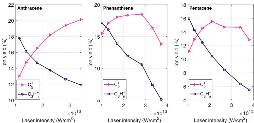
FIG. 7. Variation of the relative yield of the ionic fragments C<sub>2</sub><sup>+</sup> and C<sub>3</sub>H<sub>n</sub><sup>+</sup> with different laser intensities
