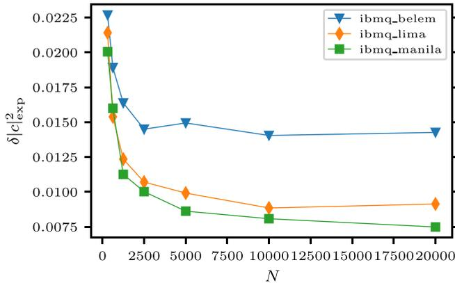
FIG. 9. Average error in measured occupation probabilities with the number of shots,  $N$ . Increasing the number of shots decreases the statistical noise yielding an estimate for the quantum computer’s measurement error. The error in the occupation probabilities yielded by these simulations are bounded from above by  $\delta|c|_{\text{exp}}^2 = 0.016$ , accounting for only a small fraction of the error observed in calculated fidelities and expectation values.
