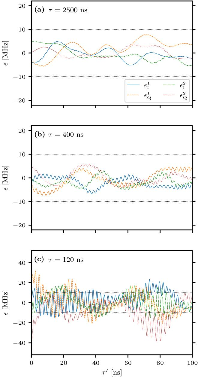
FIG. 4. First 100 ns of the control pulses with lengths (a)  $\tau = 2500$  ns, (b)  $\tau = 400$  ns, and (c)  $\tau = 120$  ns realizing the first unitary in the sequence of Eq. (12). The dependence of the amplitude of the control pulse on its length sets a lower bound for the implementation time of two-qubit gates on present-day quantum devices.
