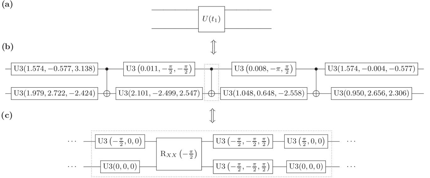
FIG. 8. Decomposition of the first short-time propagator in Eq. (12) [circuit (a)] into CNOT and U3 gates [circuit (b)]. Circuit (c) shows the decomposition of the CNOT gate into elementary gates.
