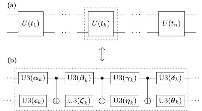
FIG. 2. Decomposition of the  $k$ th unitary transformation in the sequence of Eq. (12) [circuit (a)] into CNOT and U3 gates [circuit (b)]. Each U3 gate depends on three Euler angles. The quantum circuit resulting from this decomposition can be directly implemented on IBMQ systems.
