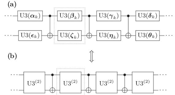
FIG. 6. Combination of simultaneous two U3 gates [circuit (a)] into two-qubit  $U^{(2)}$  gates [circuit (b)]. The CNOT and  $U3^{(2)}$  gates in circuit (b) are realized with control pulses for which the combined lengths match the implementation time of circuit (a) on IBMQ systems.
