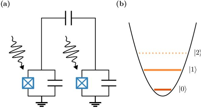
FIG. 3. Schematic representation of (a) the model two-qubit processor, consisting of two capacitively coupled superconducting transmons controlled with microwave pulses, and (b) the energy spectrum of a superconducting transmon in which the lowest two levels, shown as solid lines, are the computational qubit.
