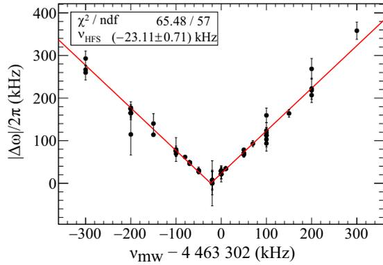
FIG. 5. Determination of  $\nu_{\text{HFS}}$  from the fitting results of the Rabi-oscillation analysis for different microwave frequencies. The data were for a krypton gas target with a pressure of about  $7 \times 10^4$  Pa.
