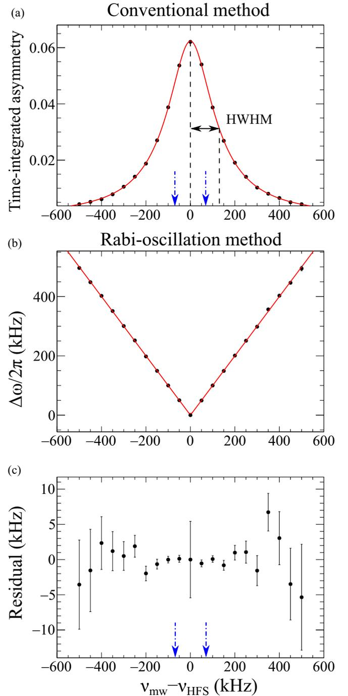
FIG. 2. Simulation results of (a) the conventional and (b) the Rabi-oscillation methods. The solid lines indicate the fitting results. (c) The residuals of the Rabi-oscillation method. The black dashed lines and the horizontal arrow in (a) indicate the HWHM of the resonance curve, and the blue dash-dotted arrows in (a) and (c) represent the detuning frequency with the lowest uncertainty in the Rabi-oscillation spectroscopy.
