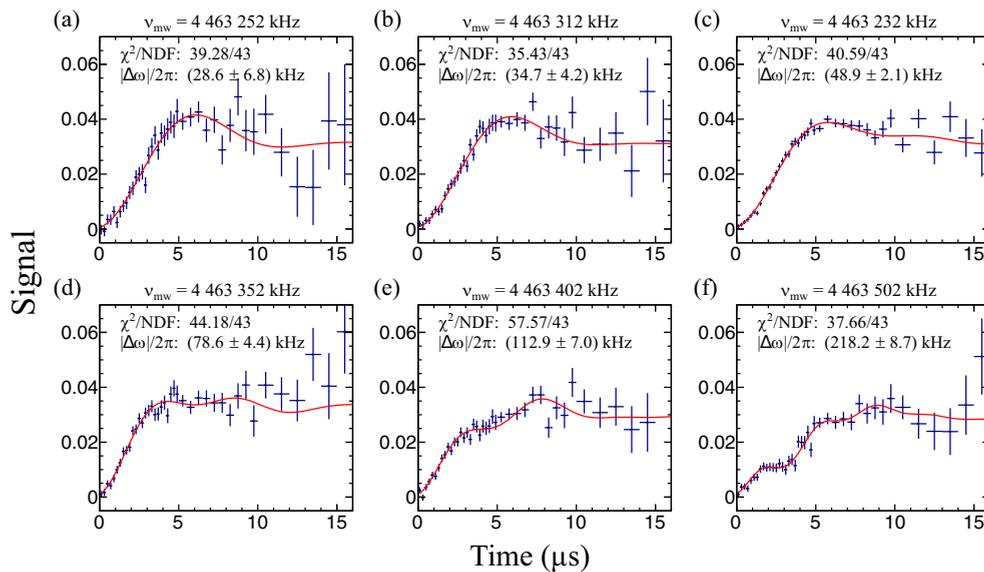
FIG. 4. Experimental results with the Rabi-oscillation spectroscopy. (a)–(f) show the time evolution of resonance signals with microwave frequencies from 4 463 232 to 4 463 502 kHz and are shown in ascending order of the absolute value of the detuning frequency  $|\Delta\omega|/2\pi$ . The solid lines indicate the fitting results.
