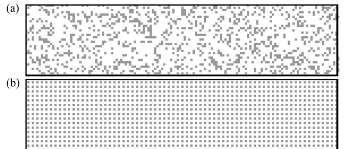
FIG. 2. The impurity potential V_{\text{imp}} is depicted for randomly (a) and regularly (b) distributed potential spikes for the same fill-factor \eta = 0.25 . Only the channel segments of the dumbbell trap are shown.
