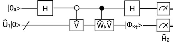
FIG. 1. Measurement scheme for terms in Eq. (25). States  $|\Phi_{\kappa_\pm}\rangle = (\hat{V} \pm \hat{W}_k \hat{V})\hat{U}_1|0\rangle / (2\sqrt{p_\pm})$  are obtained after measurement of the ancilla qubit, where  $p_\pm = \langle 0|\hat{U}_1^\dagger(\hat{V} \pm \hat{W}_k \hat{V})^\dagger(\hat{V} \pm \hat{W}_k \hat{V})\hat{U}_1|0\rangle/4$  is the probability for the ancilla qubit results to be  $\pm 1$ , respectively. H is the Hadamard gate.
