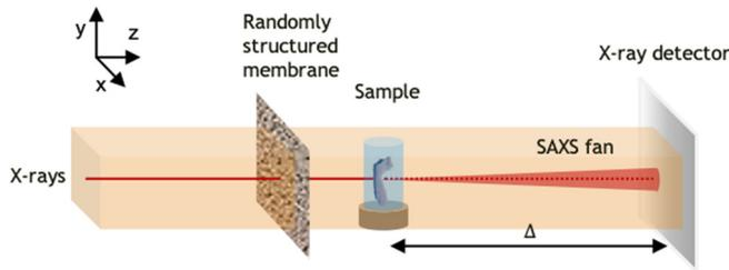
FIG. 1. Experimental setup for x-ray MIST.
