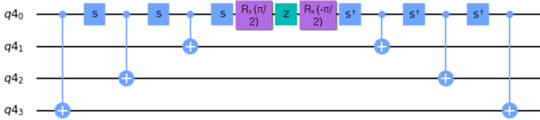
FIG. 8. Sequence of gates that implement the beam-splitting interaction term U_{+-}^1 for \frac{\epsilon_{+-}}{8} = \frac{\pi}{2} . The order of the qubits is the same as in the text.
