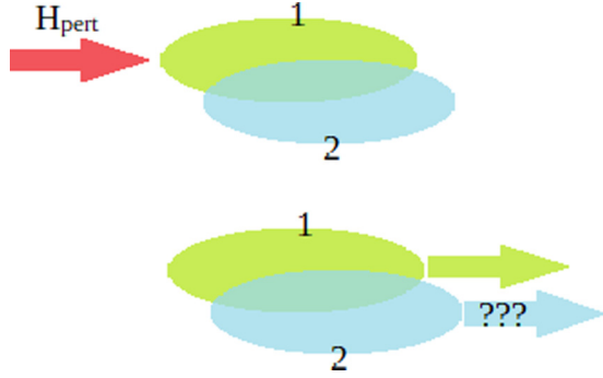
FIG. 1. Schematic visualization of fast spin drag. A fast kick, applied to the component 1 of a mixture, can drag the motion of the component 2.
