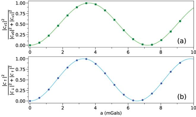
FIG. 2. Simulated measurement of  $\sin^2(\frac{\Delta\phi_Q}{2})$  vs a small background acceleration  $a$  using TAI with scalar (a) and spinor (b) wave functions. Squares and dots in (a) and (b) are from wave-function simulation data, while solid lines are semiclassical path-integral data. No fitting is performed.
